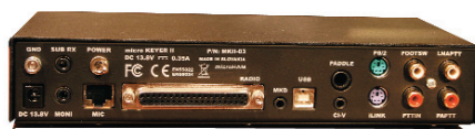
The rear panel is fairly uncluttered. Transceiver-specific interface cables plug into the large D socket.
